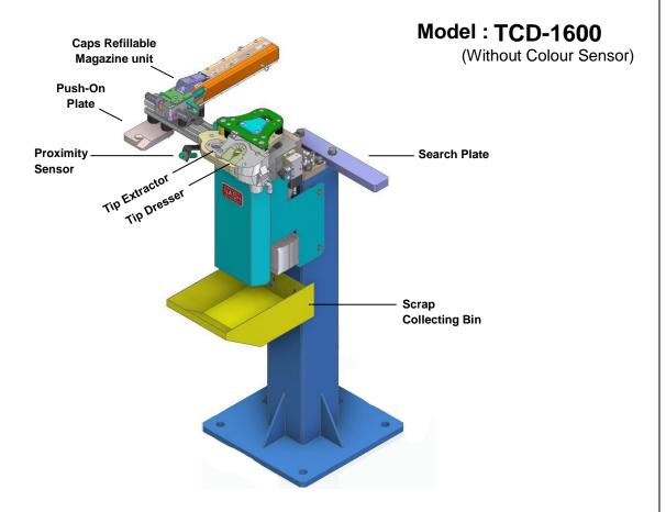
After the welding tips are worn out, **Auto tip Changing cum Dresser** will automatically perform as under –
