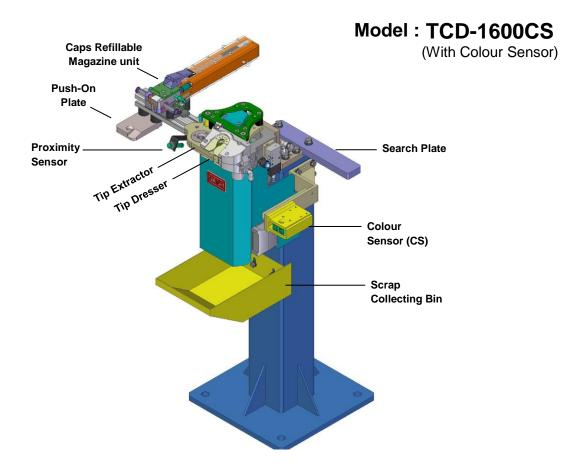
After the welding tips are worn out, **Auto tip Changing cum Dresser with Sensor** will automatically perform as under –
