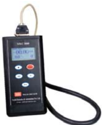
Digital Weld Monitor (Reset Box) with optional job counter for easy monitoring and programming of spot count and job count from weld monitor itself.
