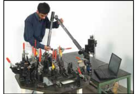
Fixture inspection by portable CMM
