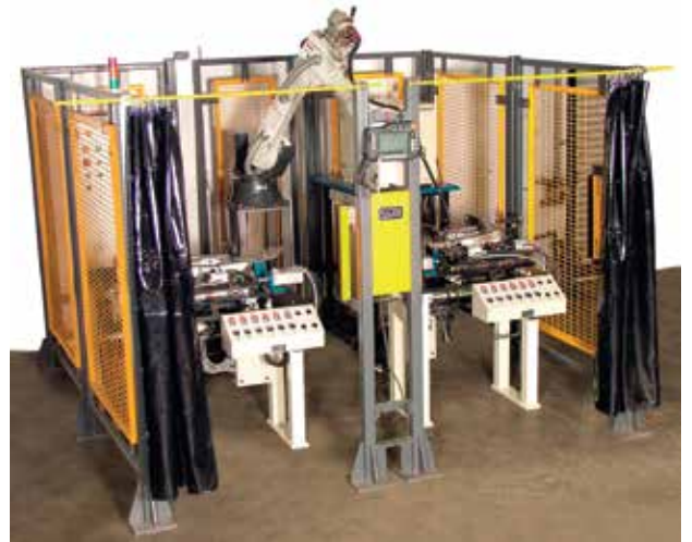
Robotic Welding Cell & Fixtures for Rear & Front Door Hinges
