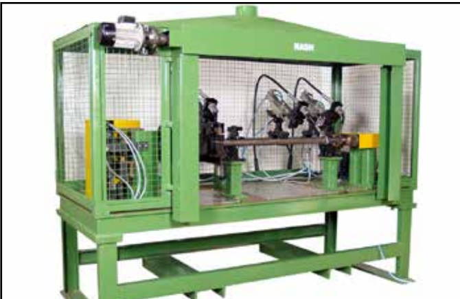
Circular Welding SPM with 03 torches for welding of output from OP-01 (OP-10)
