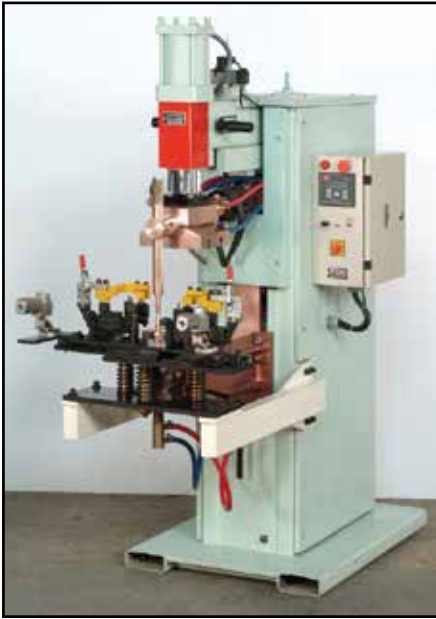
Spot Welding Machine with self equalising tooling
