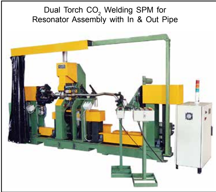
Horizontal SPM for circular welding of exhaust converter
