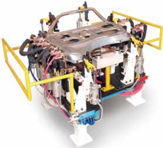
Auto Multispot (06 spot) Welder System for Door after Hemming Operation.
