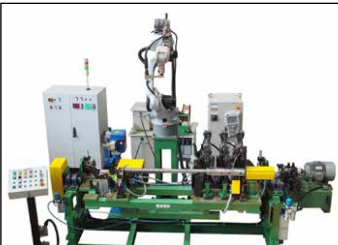
Robotic CO2 Welding fixture with Hydraulic clamps (+ Pneumatic turn table) for output of OP-10+SMBC tube (OP-20)
