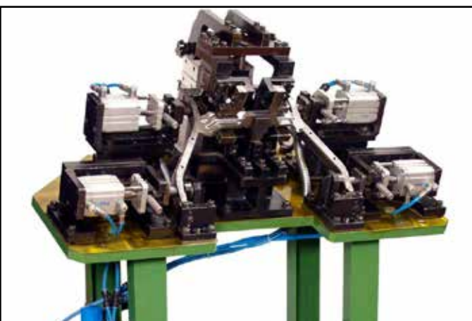
Manual Tack welding fixture for Centre Lug Assembly (OP-30)
