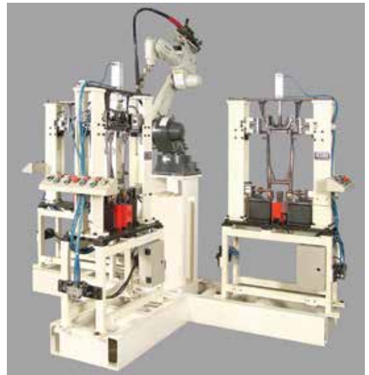
ROBOTIC WELDING AUTOMATION For TWO WHEELER SWING ARM ASSEMBLY
