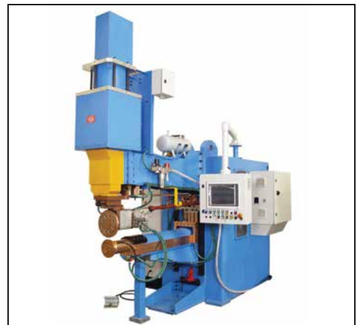
Inverter (MFDC) 600 KVA Aircraft Seam Welding Machine
