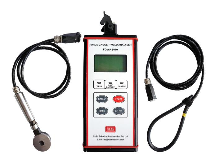
The **Force Gauge cum Weld Analyser** is microcontroller-based compact & lightweight instrument for accurate measurements of Electrode Forces and Weld Currents.
