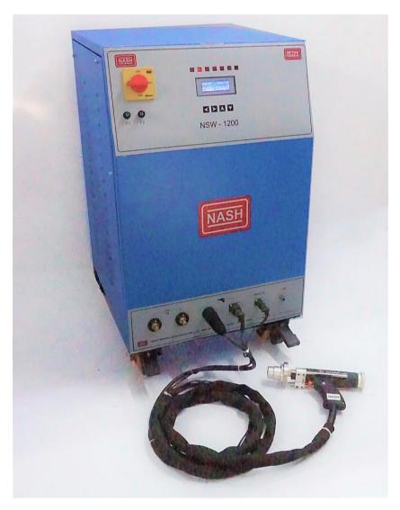
NASH 'NSW-HDT-1200SSM' Drawn Arc Stud Welder is one of the most advanced and versatile microprocessor-based state-of-the art technology in drawn arc stud welding. The various facilities incorporated in the controller provide precise control of the welding parameters for the achieving a good quality weld. The entire programming being carried out by four keys and a four line 20 – character backlit LCD display.
