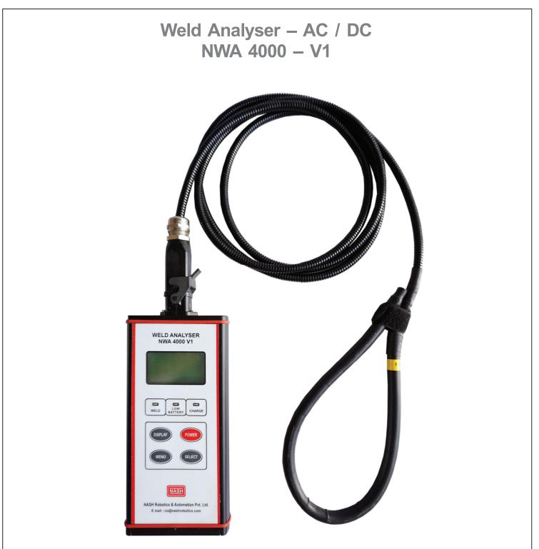
The **NASH Weld Analyser** is a microcontroller Based Compact, lightweight, hand-held, battery powered unit designed for comprehensive real time monitoring of Resistance Welds.
